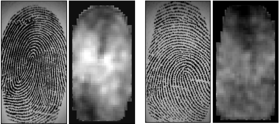
Fig. 10. Two fingerprint images and the corresponding frequency image computed with the method proposed by Maio and Maltoni [20]. Light blocks denote higher frequencies. It is quite evident that significant changes may characterize different fingerprint regions and different average frequencies may result from different fingers.
