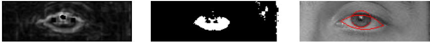
Fig. 2. Eye image processing: \phi_e obtained from the u plane; \phi_i obtained binarizing the u plane; Final result.
