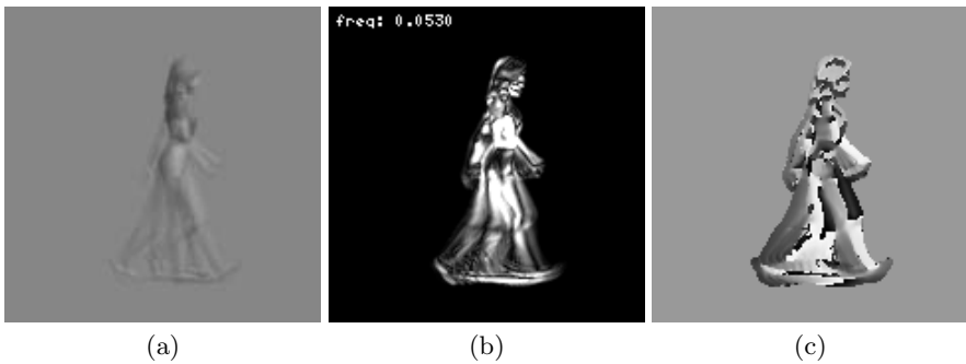
Fig. 13. Sample output of phase-locked loops: (a) superposition of frames from the input sequence, (b) magnitude of oscillations, and (c) phase of oscillations (note the phase wrap that results from the display of phase as a gray level).
